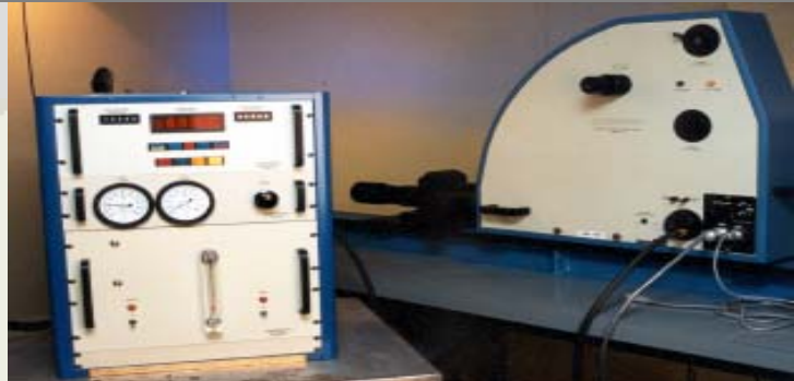
Cordin Camera Streak/framing camera with a framing rate in excess of 2.5 million frames per second.
